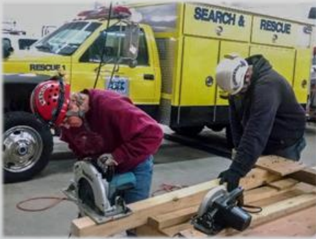
Building shoring practical in the barn. Cutting table with cleats to hold large beams for cutting.
