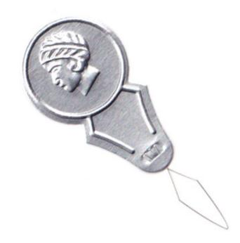
A tool that combines a short length of fine wire bent into a diamond shape with one corner held by a piece of tinplate or plastic. It is used to thread machine or hand needles.
