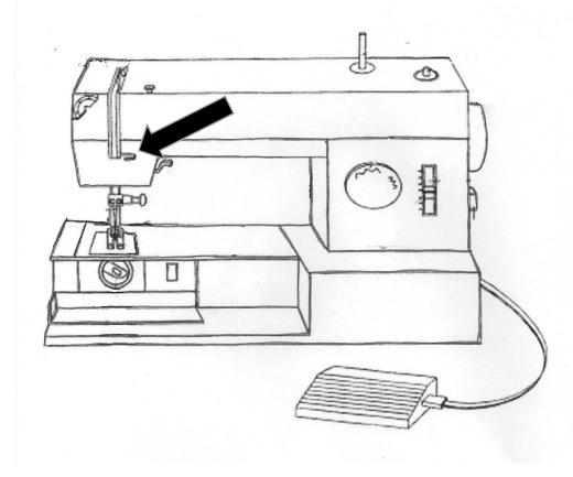
• This part directs the flow of thread to keep it going straight in one direction.
