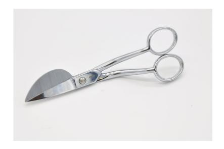
A tool that has a blade with a rounded part on one side that serves as a safety precaution to keep from cutting the base fabric. It gives the ability to precisely trim along seem lines and around edges.
