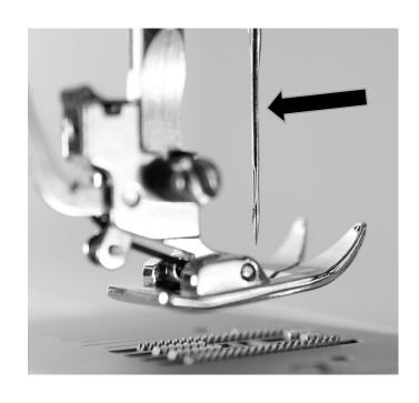
This part consists of a shank, shoulder, shaft, groove, scarf, eye, and point and is used to form stitches.
