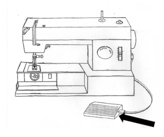
This part is placed on the floor and used to control the speed of the machine.
