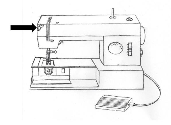
This part sets the balance between the bobbin and needle threads to determine how tight the stitches are.
