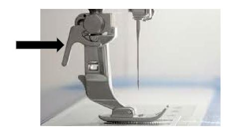
• This part is used to lower or raise the presser foot.
