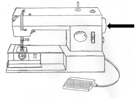
This part is used when you want to manually move the needle up and down. You must always pull it towards yourself to prevent tangling of the threads. It can be pulled out when you want to disengage the needle (run the spool of thread without the needle going up and down).
